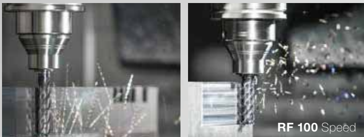
Chip formation using a conventional end mill (left) versus the RF 100 Speed (right).
